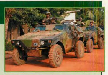
from nuclear and bio-chemical weapons attack. An interesting feature of the VBL is that it can float and, using a propeller built into the rear of the chassis, the vehicle can navigate across bodies of water at a speed of 5 knots.
